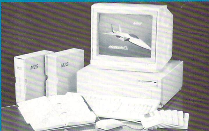
A2000 & M2Sprint Development System with Programmer's and Library Ref. Manuals and six release disks
